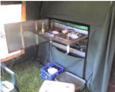
A kitchen can slide out or the tailgate can be opened through the opening in the tent panel at the back of the trailer.
